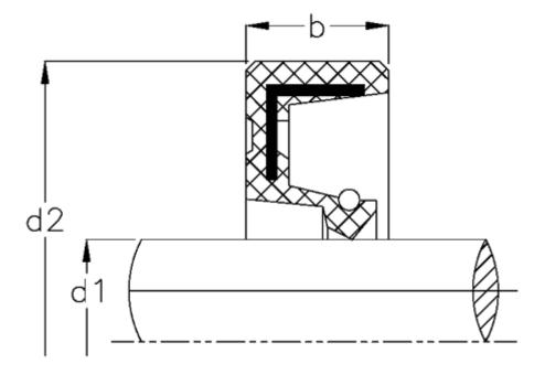
$\begin{array}{ll} b & = 10 \\ d1 & = 32 \\ d2 & = 55 \\ Material = NBR \end{array}$
